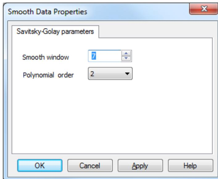
The application uses a Savitsky-Golay algorithm. Use the 'Smooth Window' and 'Polynomial Order' functions to change the degree of smoothing. Pressing 'Apply' performs the change and 'OK' completes the operation. You can use the zoom function to see more closely the effect of the smoothing. You will be asked if you want to accept the resulting smoothed spectrum.
