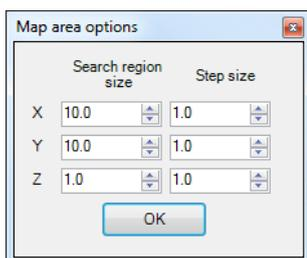
Click **OK** to display the 'Map measurement setup' window. This window should be familiar to the user as the 'Range' & 'Acquisition' tabs are identical to those in the 'Spectral acquisition setup' window (see TM004).
