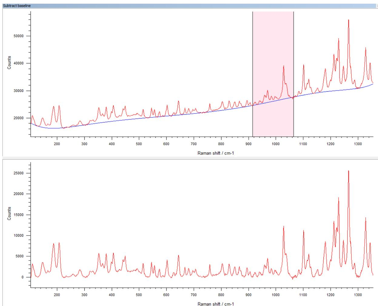
Intelligent fitting can be applied to single spectra and multfiles (e.g. mapping dataset). The baseline will automatically 'fit' each spectrum within the multfile.
