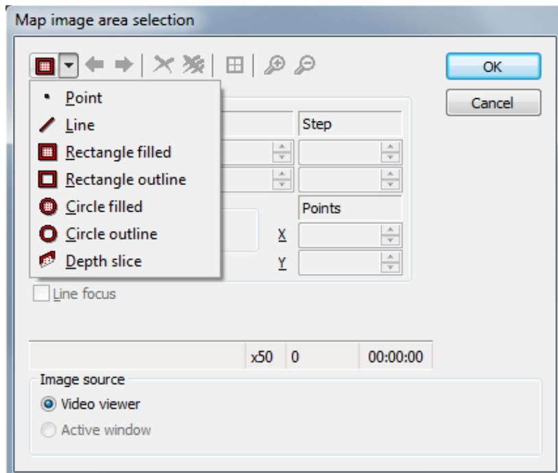
**Point** – The user can define multiple points on the base image; analyses will be performed sequentially. The XY co-ordinates are reported in the Map Image window. The blue arrows cycle through the points. The z value is fixed for each point.
