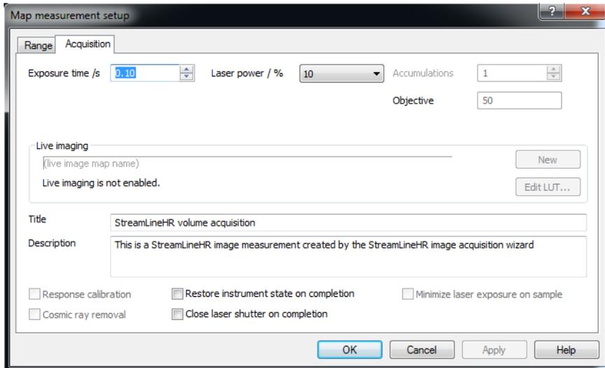
Set all parameters within this window, ensuring a suitably low laser power is selected to prevent damage to the TERS tip, & click **OK**. The 'WiRE Hotspot Mapping' viewer will automatically open. To readjust measurement settings click the 'Setup Measurement' button in the 'Settings' section of this viewer.
