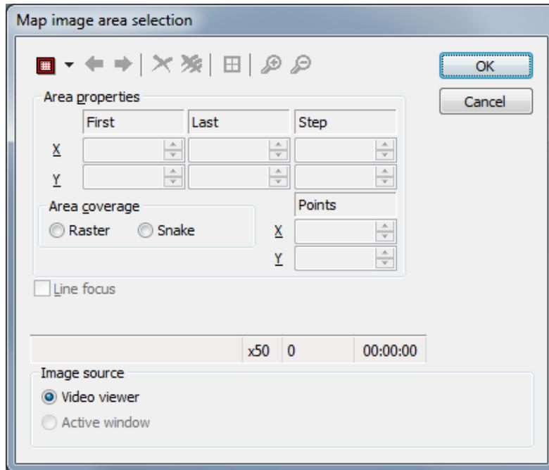
By default, the Image source is the live video viewer. A map can be defined over a larger area using a previously created montaged image. (To create a montaged image, please refer to module TM7.) If the active window contains a montage, the 'Active window' button will now be active in the Map Image window. Select it to use the montage image to define the mapping area.
