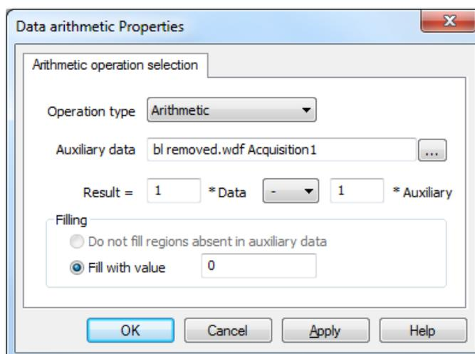
It can be useful to multiply either the sample file or the auxiliary file by a factor so that the Y axes are comparable. In the example below, 1\* the sample file and 2\* the background correction file have been used to remove the baseline. **Accept** the change either from the context menu or by closing the window.
