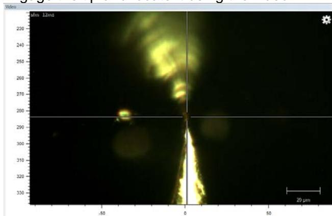
2. Focus the laser light onto the tip apex.
